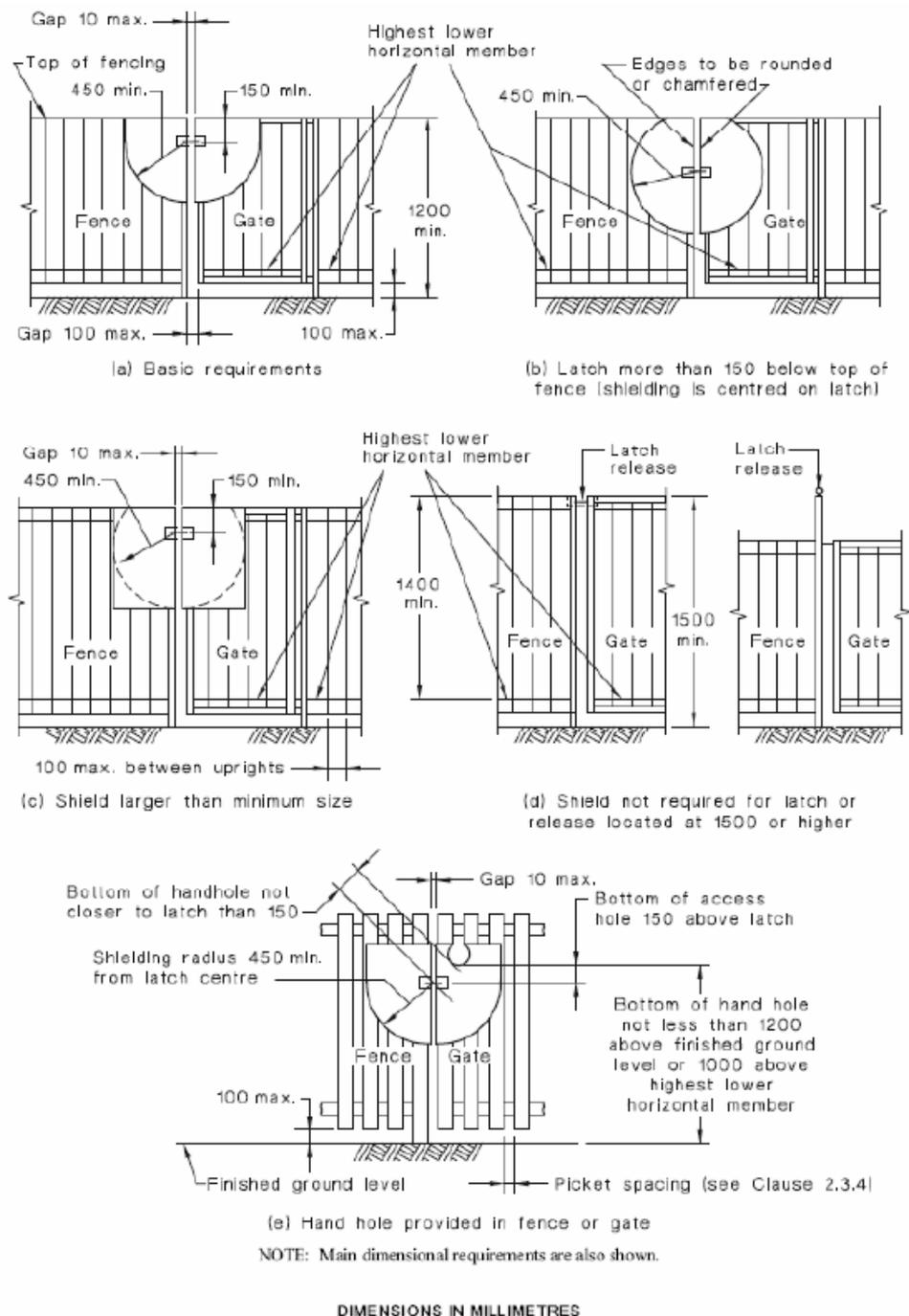
FIGURE 2.6 ALTERNATIVE LATCH SHIELDING OPTIONS FOR GATES OF OPEN CONSTRUCTION
