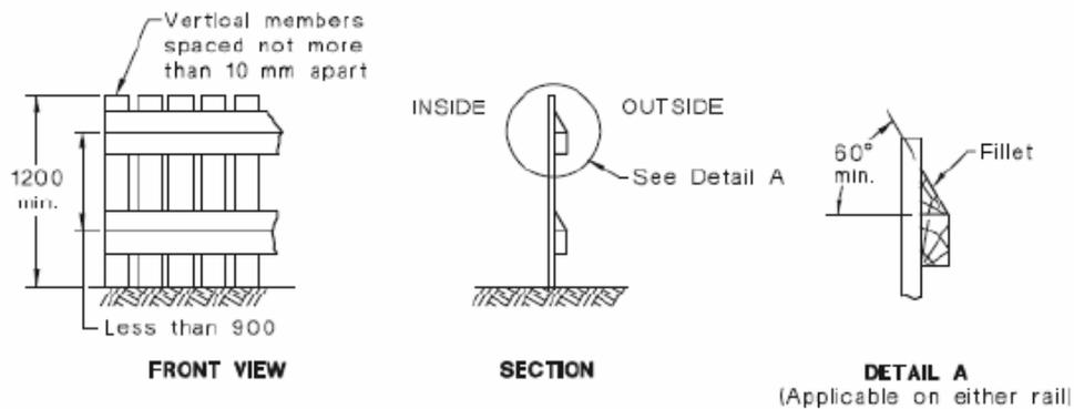
FIGURE 2.4 FENCE WITH HORIZONTAL MEMBERS PROJECTIONS OR INDENTATIONS NOT ACTING AS A HOLD FOR CLIMBING
