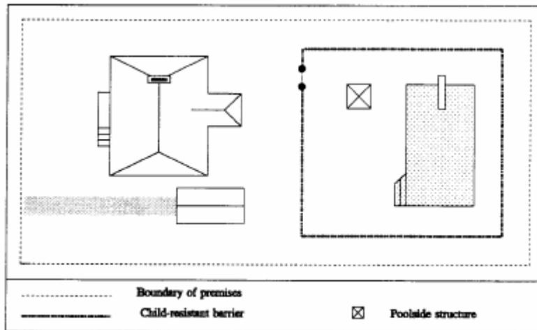
Figure 4: Boundary fencing used together with a fence to isolate the pool from the dwelling.
