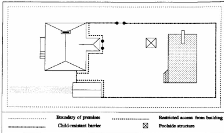
Figure 6: Existing Swimming pools and new swimming pools on very small properties (i.e properties with a site area less than 230 square metres)
