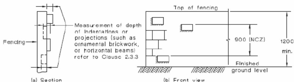
NOTE: The 900 NCZ may be between any two (2) points at any level on the outer face of the wall.
