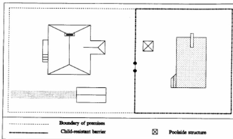
Figure 5: Existing swimming pools and new swimming pools on very small properties (i.e properties with a site area less than 230 square metres).
